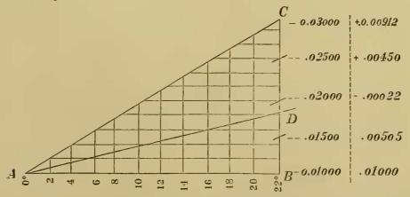
These equal distances may represent seconds, or tenths of a second. The distance  $B \ C$  is made equal to the maximum correction rm, or the correction for the maximum zenith distance, and maximum value of log.  $\rho$ , which
